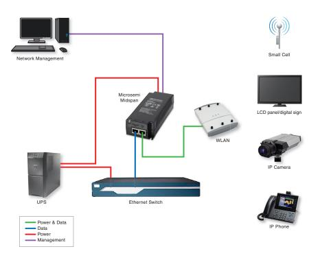
Microsemi single and multiport midspans are an economical and easy way to power popular devices such as WLAN access points, IP video phones, IP security cameras, security access devices, thin clients and printers over new or existing Ethernet infrastructure.
