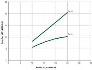
**Note:** Chart represents the range of Drop-Out, min to max, for a given Pull-in value of the MDSR-10 prior to modification into the MDSM-10.
