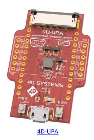
The 4D-UPA minimizes the connections and modules required for programming—creating a single module with microUSB interface, and DIP style pads for GPIO breakout of all the signals used on the gen4 Display interface, which is useful for development or final product use.
