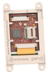
The image below (2.4" model depicted) shows a mock Application PCB on the back of the gen4 display (Blue area). It features a cut-out in the PCB so access to the micro-SD socket on the gen4's display board is possible, however this may or may not be required depending on the application and if the micro-SD socket is utilised or requiring access once the Application PCB is applied.
