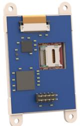
The micro-SD socket is a latch type, so it is accessible from the top, rather than a push/push or push/pull style which is accessible from the side.
