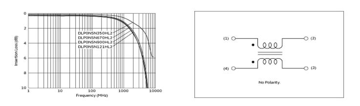
Differential Mode Transmission Characteristics (Typical Value)
