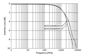
**Differential Mode Transmission Characteristics** (Typical Value)
