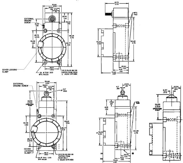
Conduit sizes 1/2-14NPT, 3/4-14NPT, M20, PG13.5, PF1/2 are available for each switch type and carry ATEX and IEC Ex approvals. 1/2-14 NPT, 3/4-14 NPT, and M20 carry UL and CSA approvals Verify that the mating threaded fitting is identical with the conduit thread shown on the product nameplate
