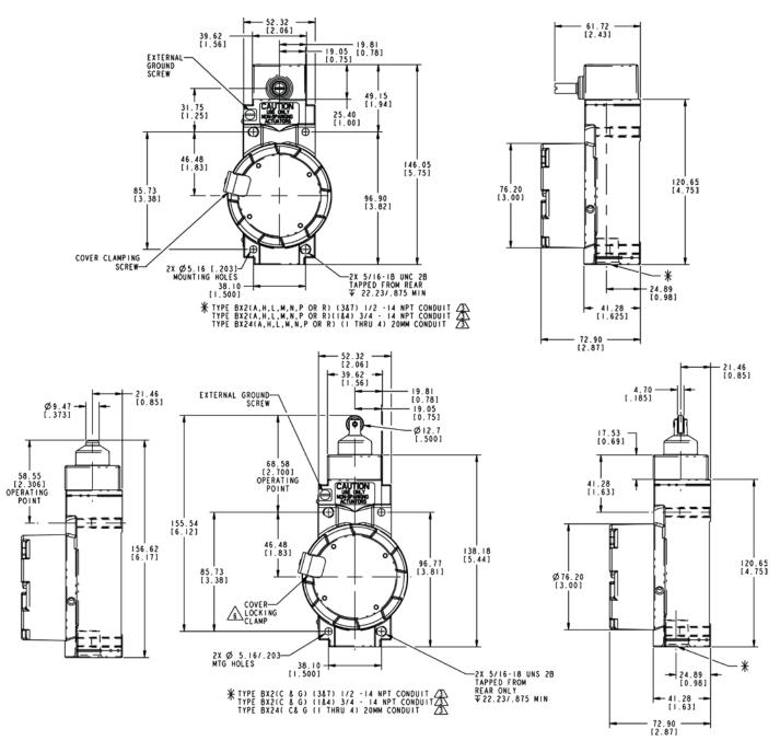
Conduit sizes 1/2-14NPT, 3/4-14NPT, M20, PG13.5, PF1/2 are available for each switch type and carry ATEX and IEC Ex approvals. 1/2-14 NPT, 3/4-14 NPT, and M20 carry UL and CSA approvals
