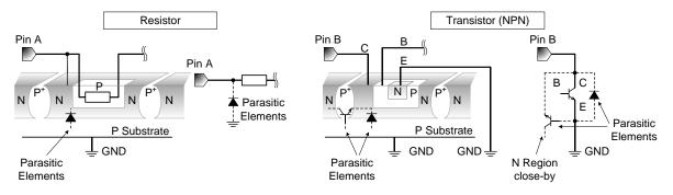
Figure 15. Example of monolithic IC structure
