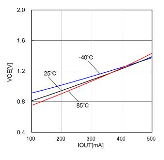
Figure 4. Output Saturation Voltage1 vs Output Current
