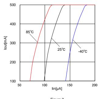
Figure 3. Output Current vs Input Current
