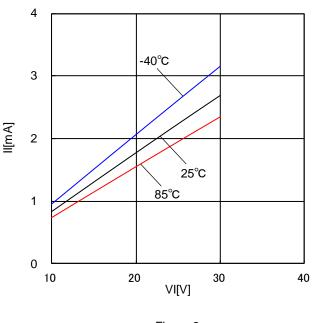
Figure 8 . Input Current vs Input Voltage (BA12004)
