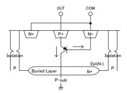
Figure 16. Construction of output clamp diode
