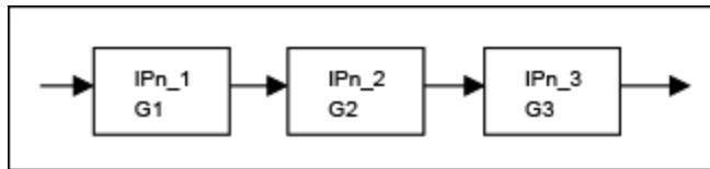
Figure 12. Cascaded RF functional blocks with known IPn.
