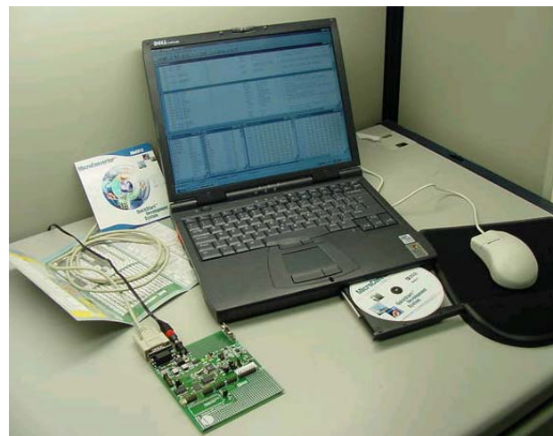
Figure 1. The ADuC8xx QuickStart Development System
