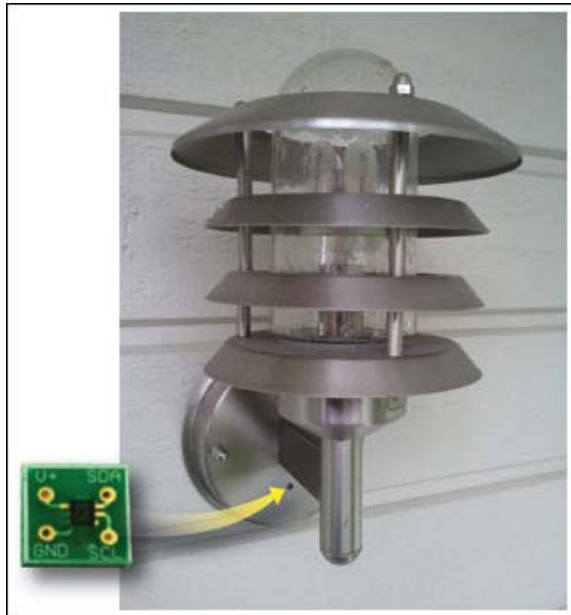
Figure 5. Ambient light sensor PCB (picture on the left) is mounted inside the luminaire chassis (small black dot visible at the bottom of the chassis). Luminaire photo courtesy of Marko Kannisto.
