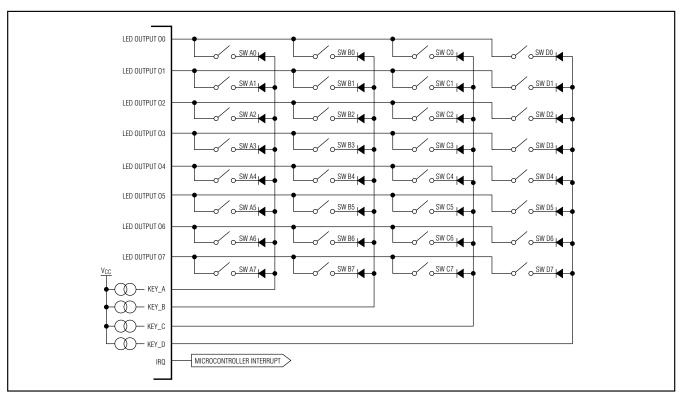
Figure 11. Key-Scanning Configuration
