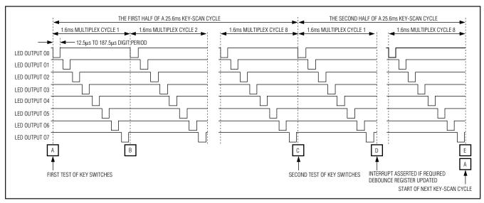
Figure 12. Key-Scan Timing Diagram
