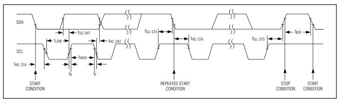
Figure 2. 2-Wire Serial Interface Timing Details
