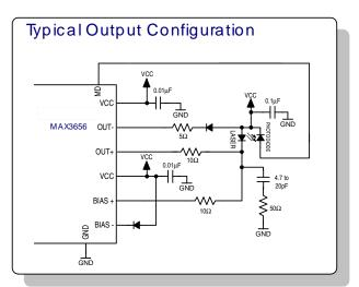
Figure 2. Typical Output Configuration
