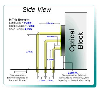
Figure 5. Lead Length Diagram (HFRD 10.2)
