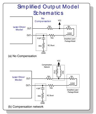
Figure 7. Simplified Output Model Schematics
