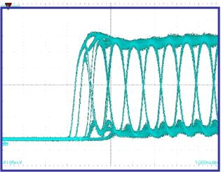
Figure 12. Burst-On Diagram with Peaking Network
