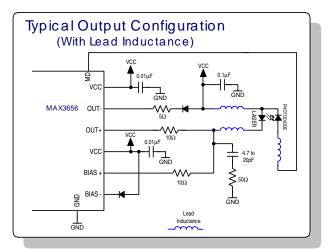
*Figure 4. Typical Output Configuration (With Lead Inductance).*
