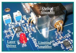
Figure 1. PCB Top Mount Laser Assembly (HFRD 10.2 Shown)
