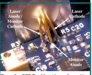
Figure 3. PCD Top Mount Laser Assembly (Laser Connection Detail)
