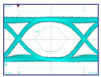
Figure 11. Filtered 1244Mbps Output With Compensation Network (>30% Margin to Standard Mask)
