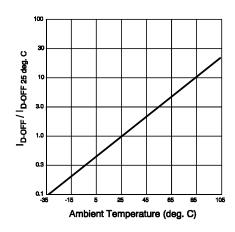
Figure 4. Typical Normalized Off-State Leakage
