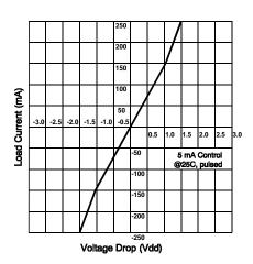
Figure 2. Linearity Characteristics
