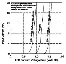
Figure 5. Input Characteristics (Current Controlled)
