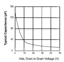
Figure 8. Typical Output Capacitance
