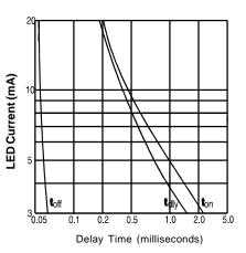
Figure 6. Typical Delay Times
