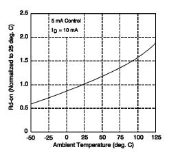
Figure 3. Typical Normalized On-Resistance
