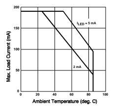
Figure 1. Typical Current Derating Curve
