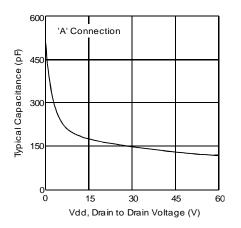
Figure 2. Typical Output Capacitance
