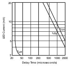
Figure 7. Typical Delay Times
