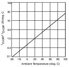
Figure 5. Typical Normalized Off-State Leakage
