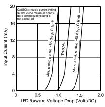
Figure 6. Input Characteristics (Current Controlled)
