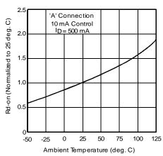
Figure 4. Typical Normalized On-Resistance
