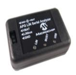
The LIN Serial Analyzer development system enables a Personal Computer (PC) to communicate with a LIN (Local Interface Network) bus as a network debug and analysis tool. The LINSA can reside on the bus as a master, slave, or non-intrusive snooper. The included PC program uses a graphical user interface to enter and display message frames occurring on the target bus.
