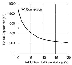
Figure 2. Typical Output Capacitance
