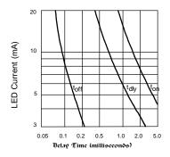
Figure 7. Typical Delay Times
