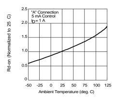
Figure 4. Typical Normalized On-Resistance
