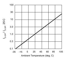
Figure 5. Typical Normalized Off-State Leakage
