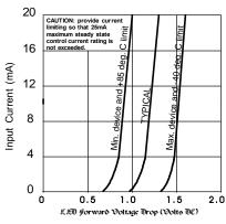
Figure 6. Input Characteristics (Current Controlled)
