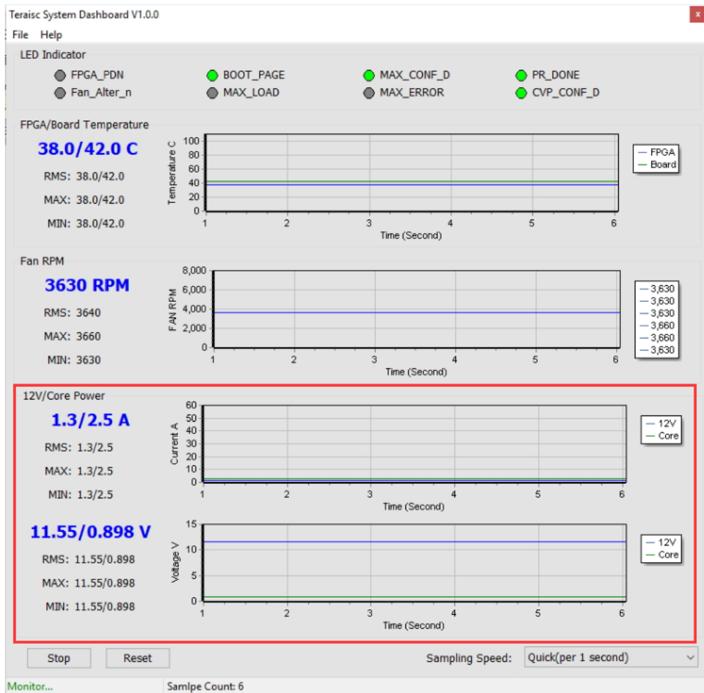
Figure 8-21 Power Monitor Section
