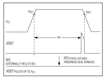
Figure 4. Battery Freshness Seal Enable Timing
