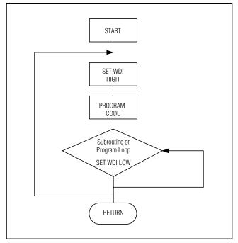
Figure 19. Watchdog Flow Diagram
