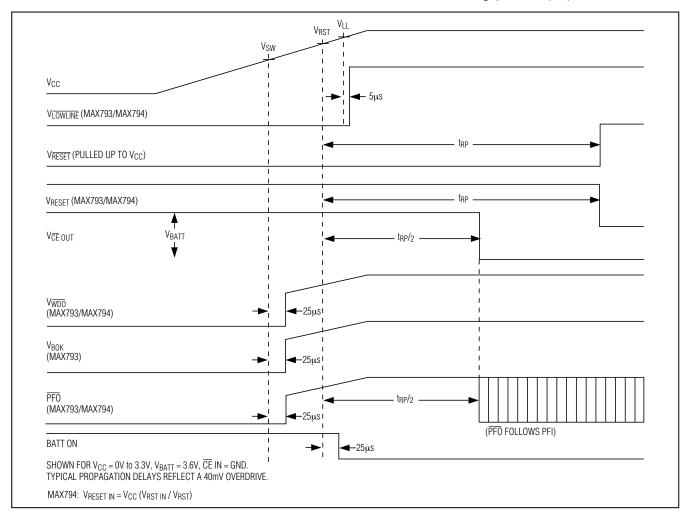
Figure 1. Timing Diagram, VCC Rising
