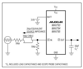
Figure 9. CE Propagation Delay Test Circuit
