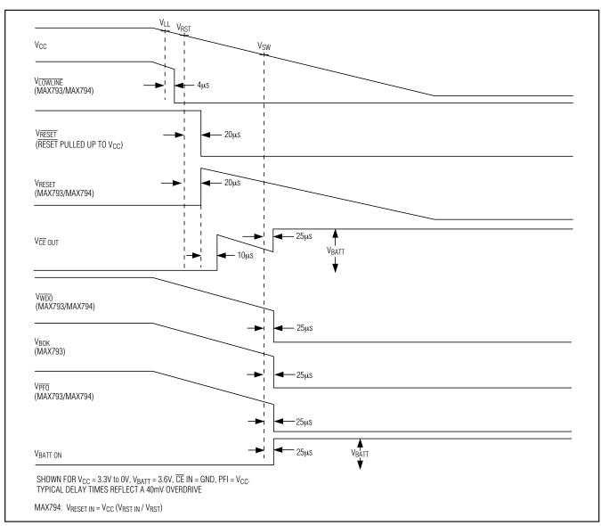
Figure 2. Timing Diagram, VCC Falling
