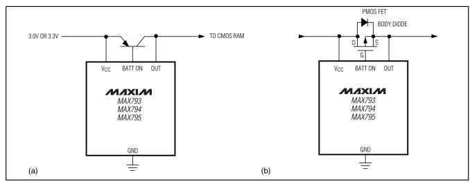
Figure 14. Driving an External Transistor with BATT ON
