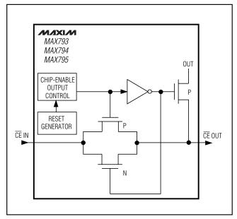
Figure 7. Chip-Enable Transmission Gate
