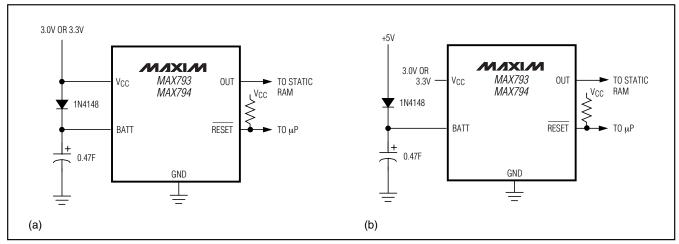
Figure 15. Using a Super Cap as a Backup Source
