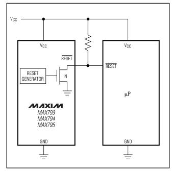
Figure 17. Interfacing to µPs with Bidirectional Reset I/O
