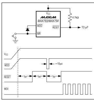
Figure 6. Generating a Reset on Each Watchdog Fault
