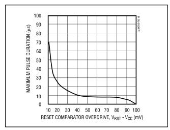
Figure 18. Maximum Transient Duration without Causing a Reset Pulse vs. Reset Comparator Overdrive
