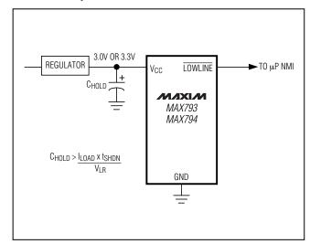
Figure 11. Using  $\overline{LOWLINE}$  to Provide Power-Fail Warning to the  $\mu P$
