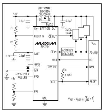
Figure 3. MAX794 Standard Application Circuit
