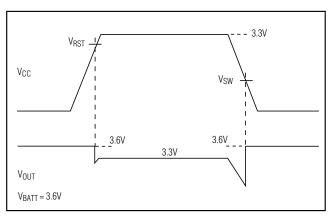
Figure 13. Battery Switchover Timing
