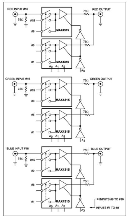
Figure 1. This multi-plane multiplexer selects any one of 16 input signals, each of which consists of the three channels R, G, and B.
