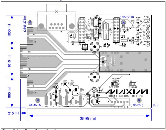
Figure 5. Host Board Dimensions / Layout
