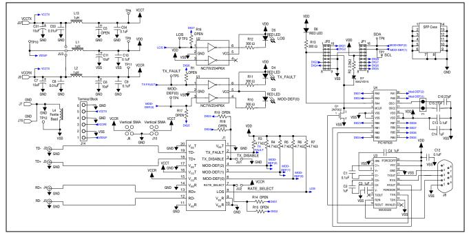
Figure 4. HFRD-15.3 SFP Host Board Schematic
