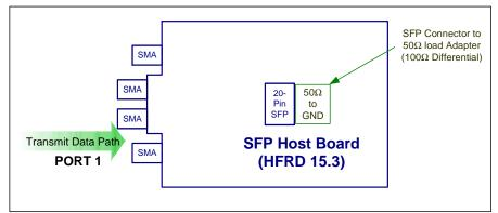
Figure 2. S11 Measurement Setup
