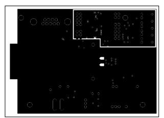
Figure 7. PC Board Layout – Ground Place
