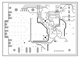
Figure 9. PC Board Layout - Solder Side
