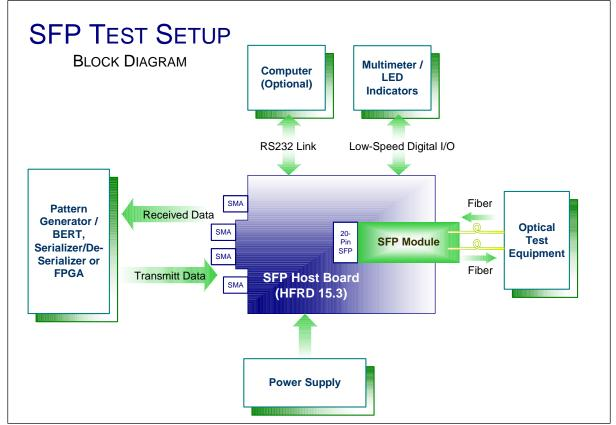
Figure 1. SFP Test Setup (Block Diagram)
