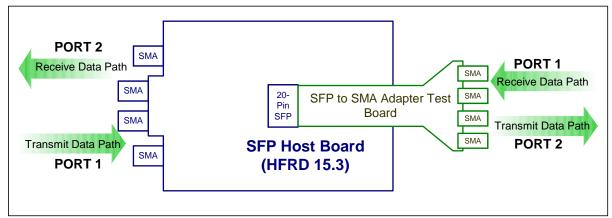
Figure 3. S21 Measurement Setup
