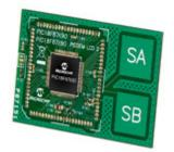
Processor Plug-In Modules are small circuit boards to be used with the various Microchip Development Boards to evaluate various MCU families. These plug into the main processor socket of the Development Boards so that different microcontrollers can be used for prototyping, demonstration or development --quickly and easily.
