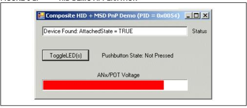
The demo PC application provides a simple graphical user interface for sending and receiving small amounts of example data to and from the HID interface on the USB device. Full source code for both this PC application and the demo firmware are included in the MCHPFSUSB Framework. Assuming the MCHPFSUSB Framework has been installed in the default location, the source code for both the firmware and PC application are found in the following directory:
