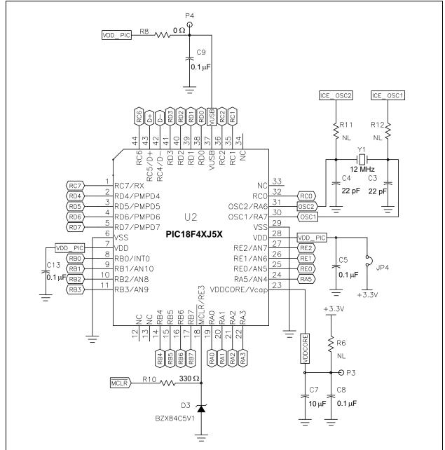
Note 1: Components, R10 and D3, are not required in production. They are included here in case the user accidentally tries to communicate with the device while a high-voltage ICSP entry device is selected in MPLAB® IDE. The PIC18F4XJ5X families use low-voltage ICSP™ entry (applying VDD levels to MCLR). High-voltage ICSP entry devices pulse the MCLR pin at around 12V when entering the ICSP mode.
