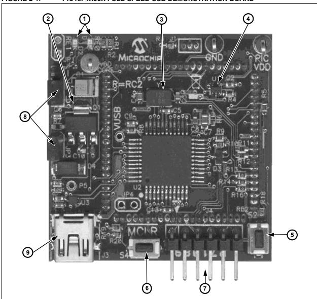
FIGURE 2-1: PIC18F4XJ5X FULL-SPEED USB DEMONSTRATION BOARD
