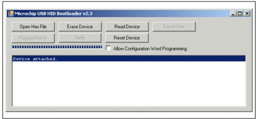
Once the PC application has found the USB device, the application can be used to open the Intel $^{\scriptsize @}$  HEX 32-bit formatted \* . hex firmware images and program them using the respective buttons.
