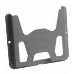
Data Pockets provide convenient storage for wiring diagrams, operation manuals and other documentation inside an enclosure. Pocket mounts on studs located on the inside of a solid-door enclosure. Constructed of high-impact thermoplastic, pockets are dark gray and have cutout areas for easy access and visibility to contents. Mounting hardware included.
