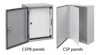
Panels swing clear from the front of the enclosure to provide access to mounted internal equipment. For CSPB panels, maximum swing is 94 degrees. For CSP panels, maximum panel swing is 106 degrees. Distance from panel surface to door when in the latched position is 1.71 in. (43 mm) for solid doors and 1.45 in. (37 mm) for window doors. Kits include panel, brackets and hardware to mount to the front flange.
