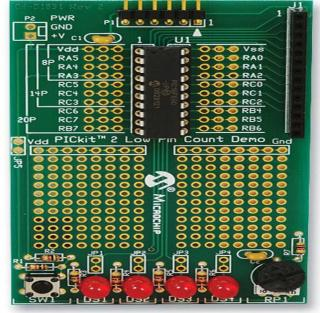
pushbutton, a prototyping area, and a 6-pin connector for PICkit 2. It also includes 2 extra bare PCB boards for your own design.
