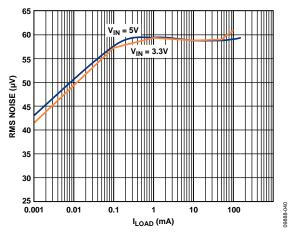
Figure 40. LDO Output Noise vs. Load Current, Across Input Voltage,  $V_{OUT3} = 3.0 V$
