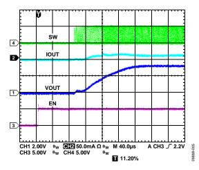
Figure 5. BUCK2 Startup,  $V_{OUT2} = 3.3 V$ ,  $I_{OUT2} = 10 mA$
