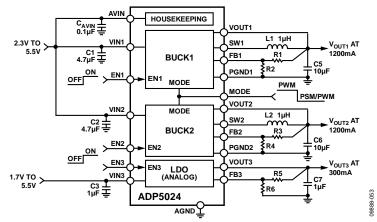
Figure 53. Adjustable Output Voltages with Enable Pins
