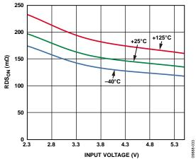
Figure 33. PMOS RDS<sub>ON</sub> vs. Input Voltage Across Temperature
