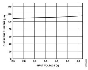
Figure 3. System Quiescent Current vs. Input Voltage, V<sub>OUT1</sub> = 3.3 V, V<sub>OUT2</sub> = 1.8 V, V<sub>OUT3</sub> = 1.2 V, All Channels Unloaded
