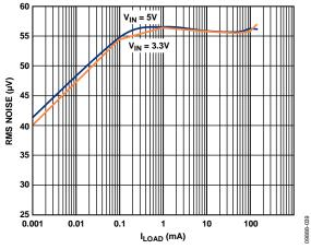
Figure 39. LDO Output Noise vs. Load Current, Across Input Voltage,  $V_{OUT3} = 2.8 V$
