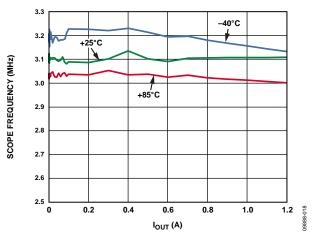
Figure 18. BUCK2 Switching Frequency vs. Output Current, Across Temperature, V<sub>0/J72</sub> = 1.8 V, PWM Mode
