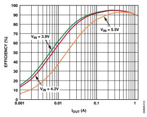
Figure 10. BUCK1 Efficiency vs. Load Current, Across Input Voltage,  $V_{\text{OUTI}} = 3.3 \text{ V}$ , PWM Mode
