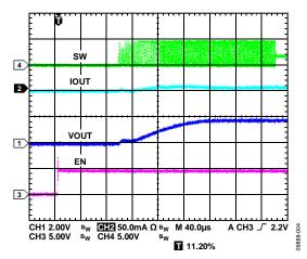
Figure 4. BUCK1 Startup, VOUT1 = 1.8 V, IOUT1 = 5 mA
