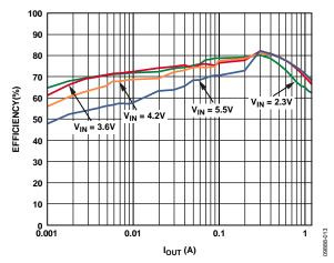
Figure 13. BUCK1 Efficiency vs. Load Current, Across Input Voltage, V<sub>OUT1</sub> = 0.8 V, Automatic Mode
