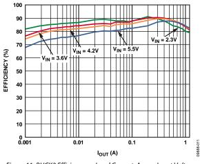
Figure 11. BUCK2 Efficiency vs. Load Current, Across Input Voltage, Vout2 = 1.8 V, Automatic Mode
