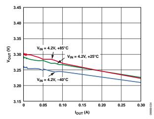
Figure 34. LDO Load Regulation Across Temperature, VIN3 = 4.2 V, VOUT3 = 3.3 V
