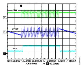
Figure 25. BUCK1 Response to Load Transient,  $I_{OUT1}$  from 1 mA to 50 mA,  $V_{OUT1}$  = 3.3 V, Automatic Mode
