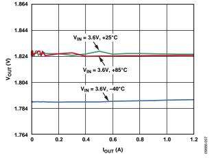
Figure 7. BUCK2 Load Regulation Across Temperature,  $V_{OUT2} = 1.8 V$ , Automatic Mode
