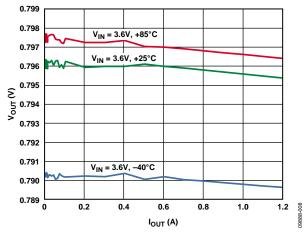
Figure 8. BUCK1 Load Regulation Across Input Voltage,  $V_{\text{OUTI}} = 0.8 \text{ V}$ , PWM Mode
