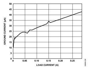
Figure 36. LDO Ground Current vs. Output Load, V<sub>IN3</sub> = 3.3 V, V<sub>OUT3</sub> = 2.8 V
