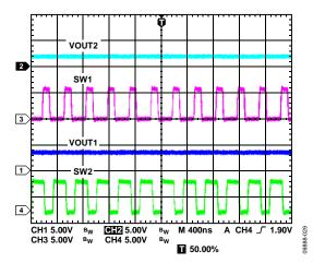
Figure 29. VOUTx and SW Waveforms for BUCK1 and BUCK2 in PWM Mode Showing Out-of-Phase Operation
