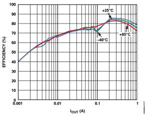
Figure 17. BUCK1 Efficiency vs. Load Current, Across Temperature, Vourn = 0.8 V, Automatic Mode
