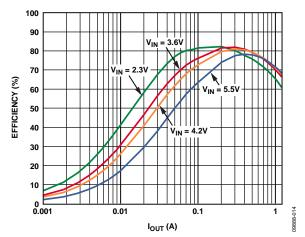
Figure 14. BUCK1 Efficiency vs. Load Current, Across Input Voltage, Vouti = 0.8 V, PWM Mode
