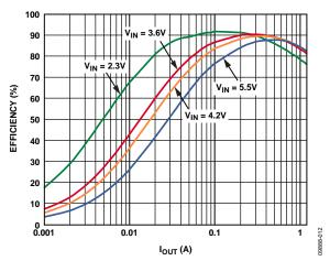
Figure 12. BUCK2 Efficiency vs. Load Current, Across Input Voltage, V<sub>0072</sub> = 1.8 V, PWM Mode
