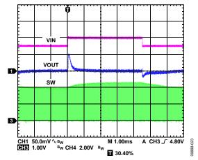
Figure 23. BUCK1 Response to Line Transient, Input Voltage from 4.5 V to 5.0 V, V<sub>OUTI</sub> = 3.3 V, PWM Mode
