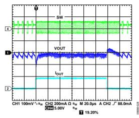
Figure 28. BUCK2 Response to Load Transient, IouT2 from 20 mA to 180 mA, VouT2 = 1.8 V, Automatic Mode
