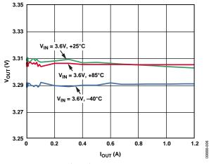
Figure 6. BUCK1 Load Regulation Across Temperature,  $V_{OUTI} = 3.3 V$ , Automatic Mode
