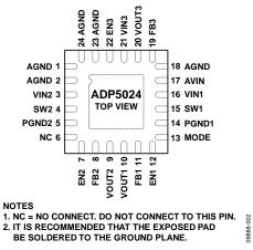
Figure 2. Pin Configuration—View from Top of the Die
