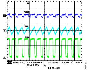
Figure 21. Typical Waveforms, Vouti = 3.3 V, Iouti = 30 mA, PWM Mode
