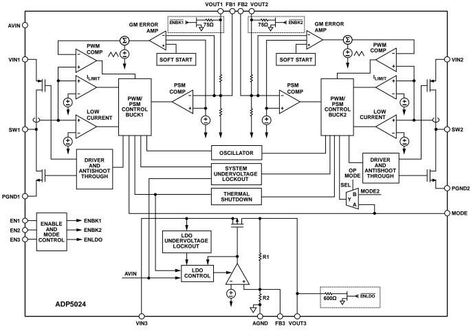
Figure 45. Functional Block Diagram
