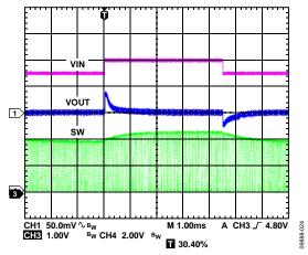
Figure 24. Buck2 Response to Line Transient,  $V_{\rm IN}$  = 4.5 V to 5.0 V,  $V_{\rm OUT2}$  = 1.8 V, PWM Mode
