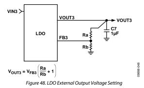
The LDO also provides high power supply rejection ratio (PSRR), low output noise, and excellent line and load transient response with only a small 1  $\mu$ F ceramic input and output capacitor.
