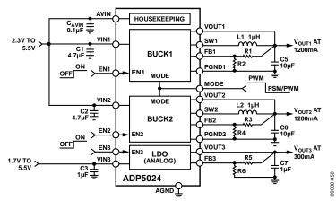
Figure 50. Processor System Power Management with PSM/PWM Control
