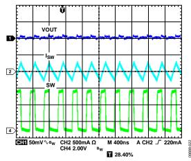
Figure 22. Typical Waveforms, Vout2 = 1.8 V, Iout2 = 30 mA, PWM Mode
