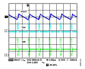
Figure 20. Typical Waveforms,  $V_{OUT2} = 1.8 V$ ,  $I_{OUT2} = 30 mA$ , Automatic Mode
