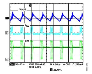
Figure 19. Typical Waveforms, V<sub>OUT1</sub> = 3.3 V, I<sub>OUT1</sub> = 30 mA, Automatic Mode
