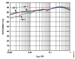
Figure 16. BUCK2 Efficiency vs. Load Current, Across Temperature,  $V_{OUT2} = 1.8$  V, Automatic Mode
