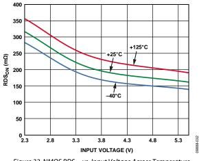
Figure 32. NMOS RDSON vs. Input Voltage Across Temperature
