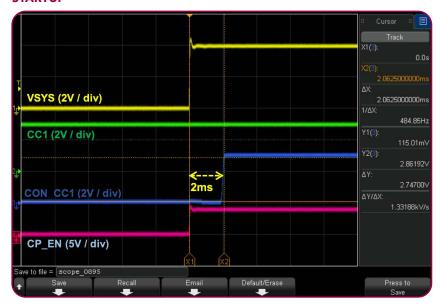
**Start up:** 2 ms power-up time from valid power source of  $V_{\rm SYS}$ . When  $V_{\rm SYS}$  is below VSYSUVLO, NX20P0477 stays in shutdown mode, where both CC switches are turned off. Once  $V_{\rm SYS}$  is above VSYSUVLO, then NX20P0477 transitions to active state by turning the CC switch on within power-up time.
