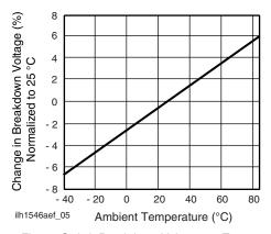
Fig. 4 - Switch Breakdown Voltage vs. Temperature
