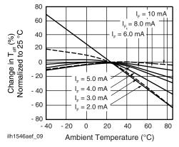
Fig. 8 - Turn-off Time vs. Temperature
