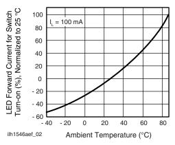
Fig. 2 - LED Current for Switch Turn-on vs. Temperature
