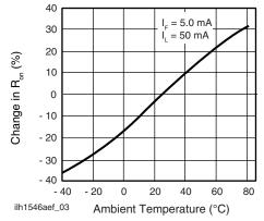
Fig. 3 - On-Resistance vs. Temperature
