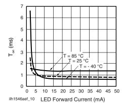
Fig. 9 - Turn-on Time vs. LED Current
