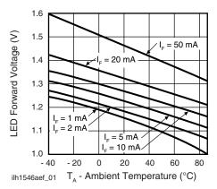
Fig. 1 - LED Voltage vs. Temperature
