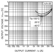
Fig.4 Output voltage vs. output current
