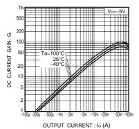
Fig.3 DC current gain vs. output current
