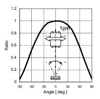
Fig.4 Directional Characteristics 1
