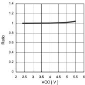
Fig.9 IOUT VCC dependency
