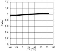
Fig.8 IOUT Temperature dependency (100 lx)
