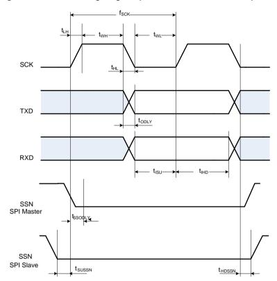
Figure 7-1. SPI Timing Diagram (SPI Mode CPOL=0, CPHA=0)
