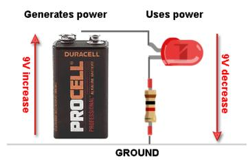
In our three-piece circuit, we have the battery (which generates voltage) and the resistor+LED (which uses up the voltage). I will now tell you a very key 'law' of electronics:
