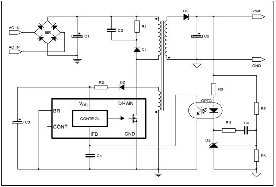
Figure 20. Min-features flyback application
