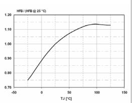
Figure 11. Brown out threshold vs T<sub>J</sub>
