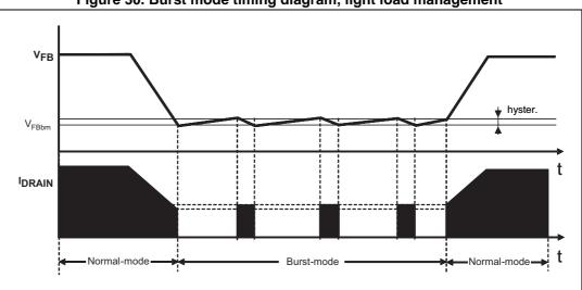
Figure 30. Burst mode timing diagram, light load management
