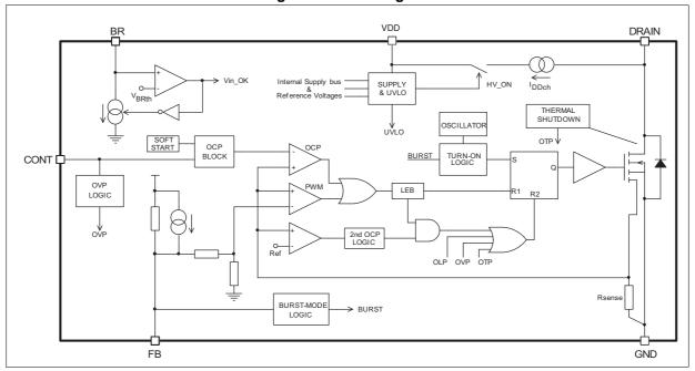
Figure 2. Block diagram
