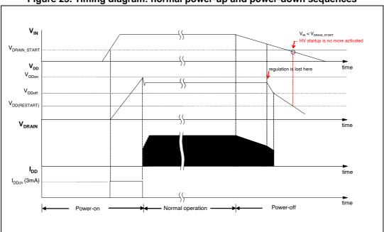
Figure 23. Timing diagram: normal power-up and power-down sequences
