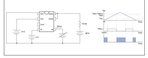
Figure 6. OVP threshold test circuit
