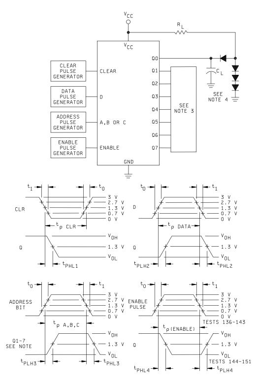
NOTE: For Q0 output waveform is inverted and tPLH3 and tPHL3 are interchanged.
