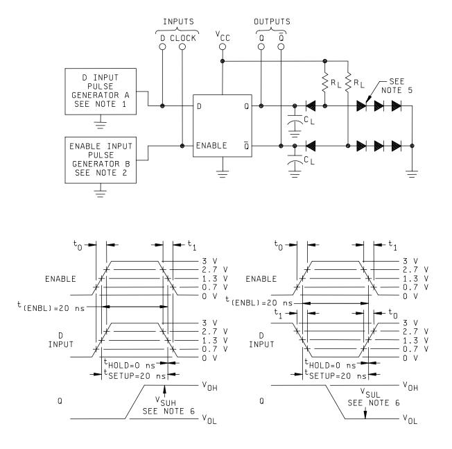
FIGURE 3. Switching test circuit and waveforms for device types 01 and 04.
