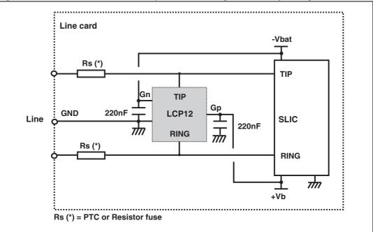
*Figure 8* shows the classical protection topology for SLIC using both positive and negative battery voltages. With such a topology the SLIC is protected against surge over  $+V_b$  and lower than  $-V_{bat}$ . In this case,  $+V_b$  can be programmed up to +120 V while  $-V_{bat}$  can be programmed down to -120 V.
