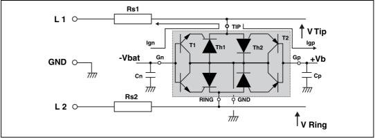
*Figure 7* shows the classical protection circuit using the LCP12 crowbar concept. This topology has been developped to protect the new two-battery voltage SLICs. It allows both positive and negative firing thresholds to be programmed. The LCP12 has two gates (Gn and Gp). Gn is biased to negative battery voltage -V<sub>bat</sub>, while Gp is biased to the positive battery voltage +V<sub>b</sub>.
