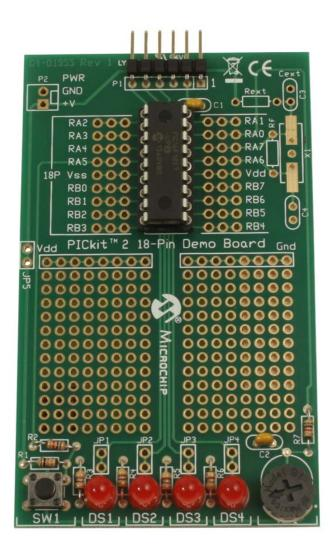
This 18-Pin Demo Board with PIC16F648A includes 4 LEDs, a potentiometer for ADC, a pushbutton, a prototyping area, and a 6-pin connector for PICkit 2. It also includes 2 extra bare PCB boards for your own design.
