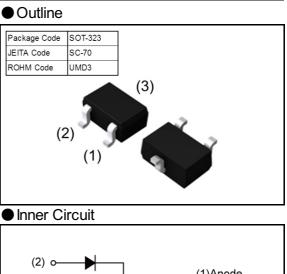
(1)Anode o (3) (2)Anode (3)Cathode (1) 0-
