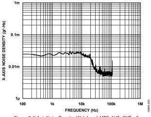
Figure 7. X-Axis Noise Density, Wideband, MTC, AVG\_CNT = 0
