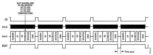
Figure 5. Burst Read Function Sequence Diagram, First Five Segments
