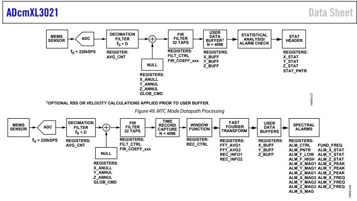
Figure 50. AFFT Mode and MFFT Mode Datapath Processing
