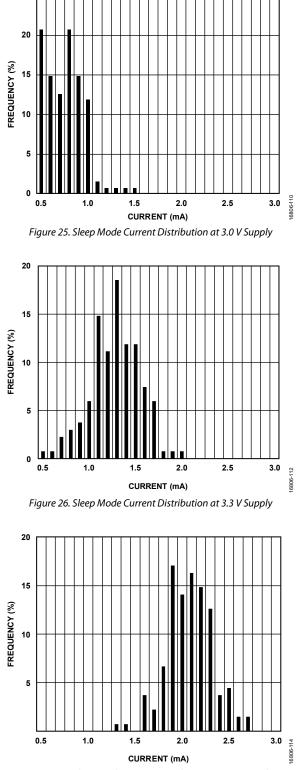
Figure 27. Sleep Mode Current Distribution at 3.6 V Supply
