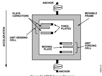
Figure 35. MEMS Sensor Diagram
