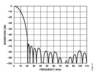
Figure 28. Digital Filter Frequency Response of the 1 kHz Low-Pass Filter
