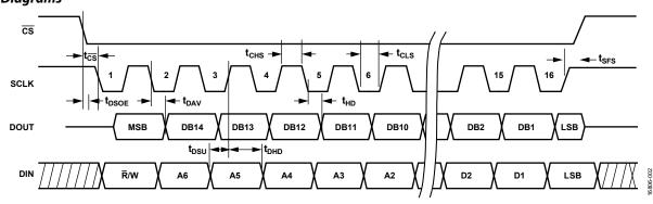
Figure 2. SPI Timing and Sequence
