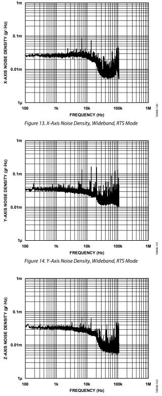
Figure 15. Z-Axis Noise Density, Wideband, RTS Mode
