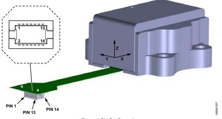
Figure 6. Pin Configuration
