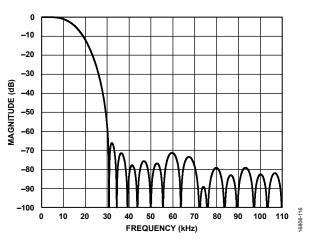
Figure 29. Digital Filter Frequency Response of the 5 kHz Low-Pass Filter
