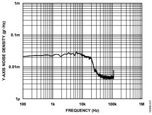
Figure 8. Y-Axis Noise Density, Wideband, MTC, AVG\_CNT = 0
