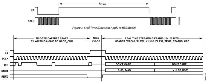
Figure 4. RTS Mode Timing Diagram (Assumes REC\_CTRL, Bits[1:0] = 0b11)
