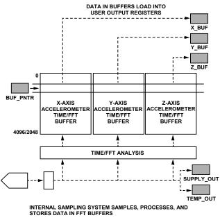
Figure 39. Data Buffer Structure and Operation
