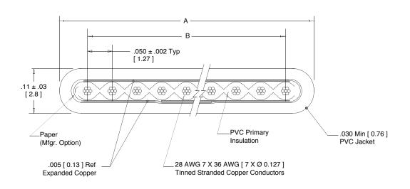
Note: Red marking on edge of primary cable designates wire #1.
