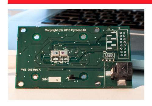
The ezPyro application specific demo kits demonstrate the capabilities of Pyreos' innovative ezPyro digital infrared sensors. The demo kits consist of a main board with up to 4 ezPyro sensors and an attached controller board based on an ARM Cortex-M4 microcontroller. There are specific kits for gas, flame, motion and gesture sensing, as well as a generic kit allowing various ezPyro sensors to be plugged into a backplane board.
