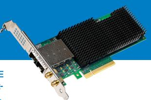
25/10/1Gb Ethernet with hardware-enhanced IEEE 1588 Precision Time Protocol (PTP) for high clock-phase accuracy synchronization across networks.
