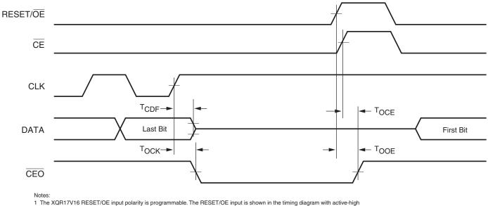
1 The XQR17V16 RESET/OE input polarity is programmable. The RESET/OE input is shown in the timing diagram with active RESET polarity. Timing specifications are identical for both polarity settings.
