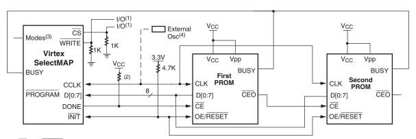
(1)  $\overline{\text{CS}}$  and  $\overline{\text{WRITE}}$  must be pulled down to be used as I/O. One option is shown.
