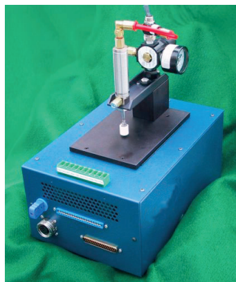
Figure 3-9: \theta_{JC} Measurement Setup
