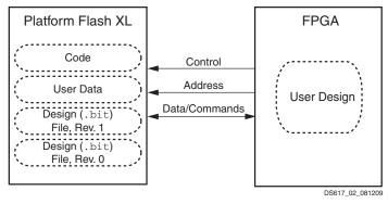
Figure 2: Standard NOR Flash Interface for User Access to Memory
