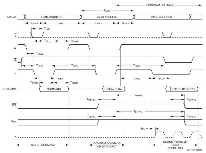
Figure 32: Write AC Waveforms, Chip Enable Controlled
