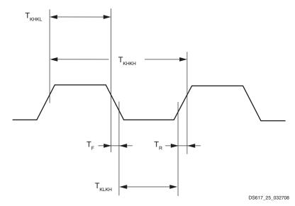
Figure 28: Clock Input AC Waveform
