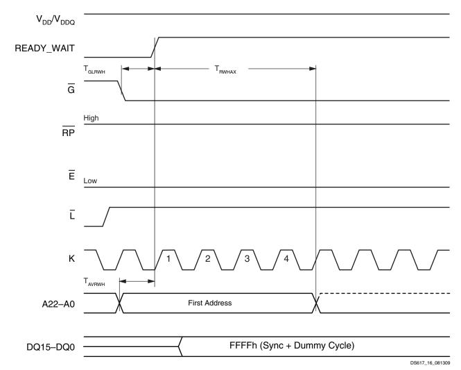
Figure 21: First Address Latching Sequence (FALS): Clock is Free Running
