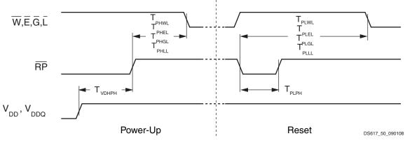
Figure 33: Reset and Power-Up AC Waveforms
