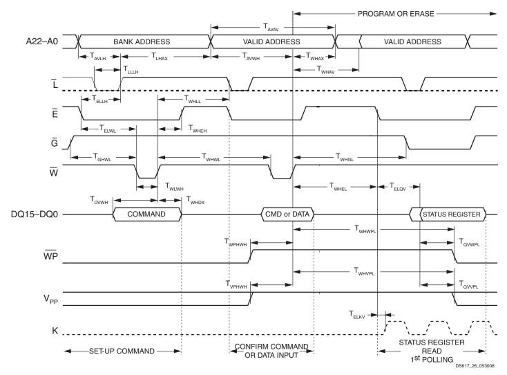
Figure 31: Write AC Waveforms, Write Enable Controlled
