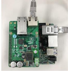
5. Connect LAN1 on PoE to LAN port on the MB with LAN cable in accessory  $% \left( 1\right) =\left( 1\right) \left( 1\right)$  kit.
