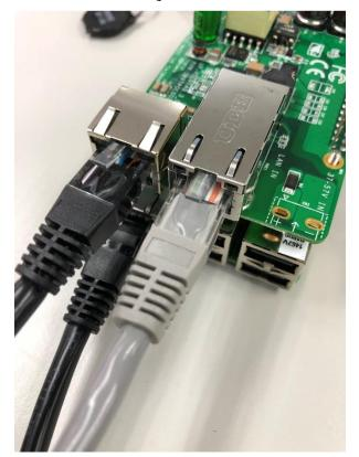
7. PoE board will power your MB through 40PIN header and transmit LAN signal to your MB via LAN cable
