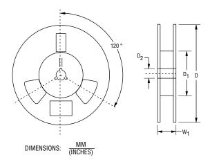
Devices are packed in accordance with EIA 481 standard specifications shown here.
