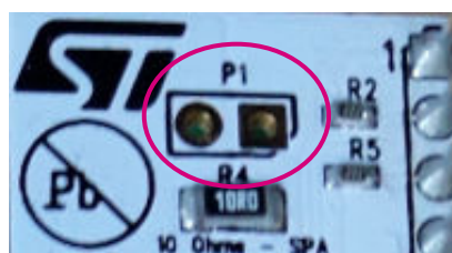
Figure 5. P1 header location
