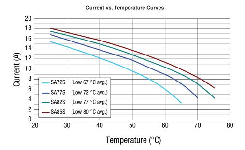
The above curves were derived from placing non-PCB mounted test samples in an oven at 25 °C, 40 °C, 60 °C, and 70 °C, increasing current flow through the sample at a rate of 0.1 A/minute and recording the current value when the sample trips. The current carrying performance is influenced by the PCB design due to copper resistance; users should verify actual device performance in their specific applications.
