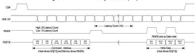
Figure 15. WRITE with 1X Latency Transaction (DDR)<sup>[20, 21]</sup>
