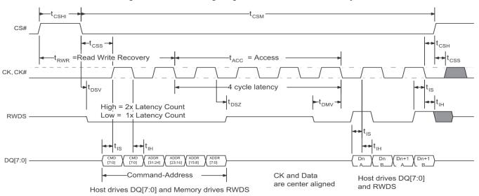
Figure 38. Write Timing Diagram — No Additional Latency
