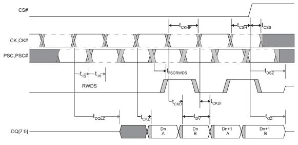
Figure 44. DCARS Data Valid Timing<sup>[57, 58, 59, 60]</sup>
