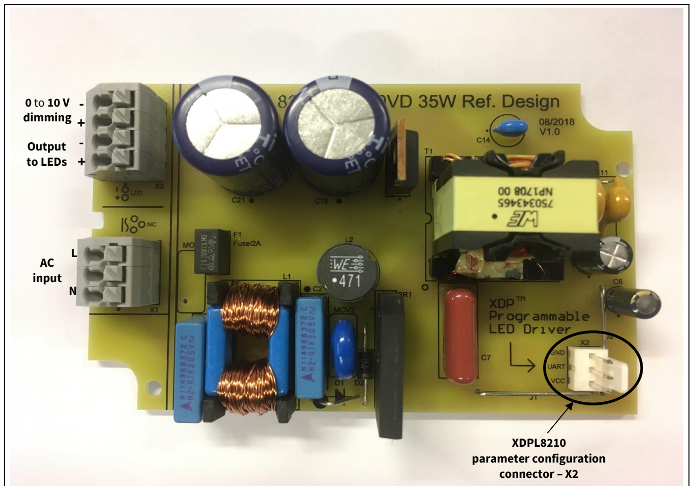
Figure 1 XDPL8210 CDM10VD 35 W reference design
