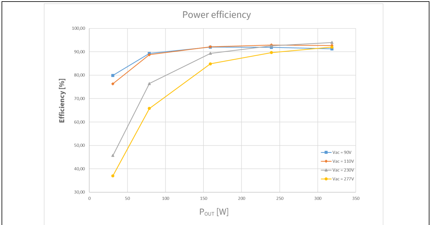
Figure 16 ICL5102 320 W reference board power efficiency measurement
